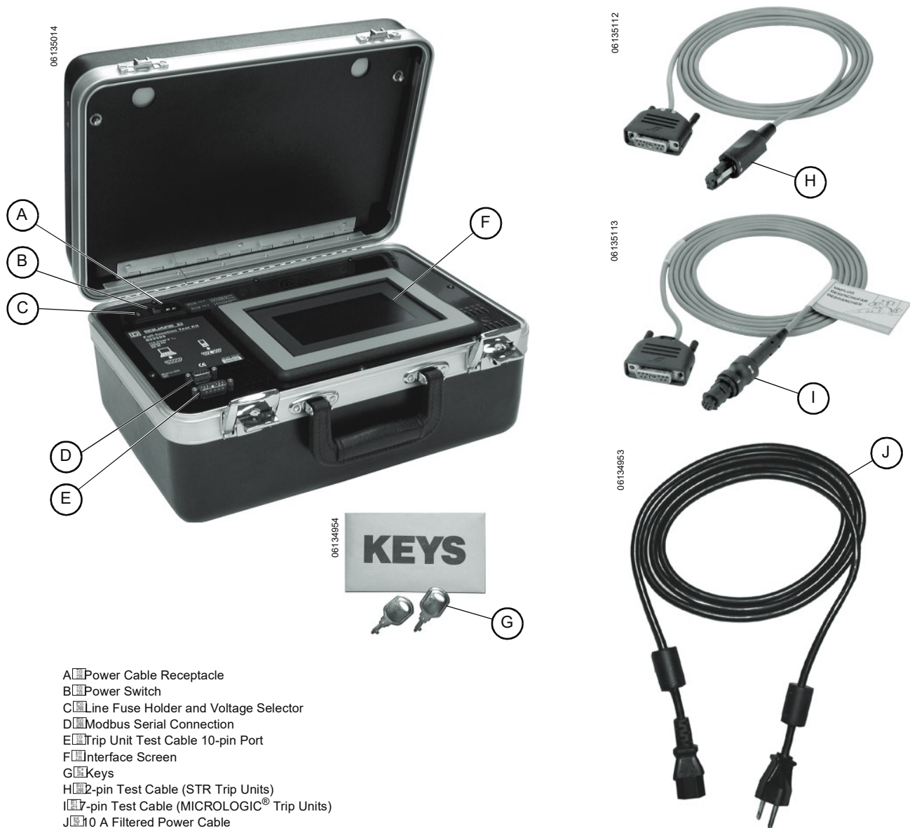
Figure 1: Full-function Test Kit and Case Contents
