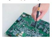
Typical applications of this magnetic field probe are evaluation of the effectiveness of a bypass capacitor located near the power supply terminal of an IC or evaluation of the microstrip layout on a PCB. Due to the probe's high spatial resolution (approximately 0.25 mm), it is not affected by adjacent patterns.
