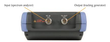
Tracking generators are ideal for tuning filters, determining the usable frequency range of amplifiers and attenuators and aligning receiver IF stages.
