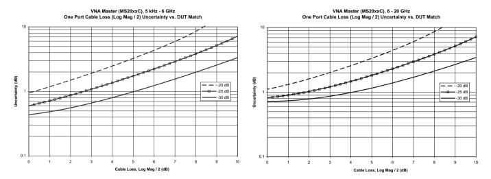
These uncertainty curves show how frequency range, DUT Match, and cable loss impact worst-case uncertainty of round-trip cable loss measurements. The uncertainty curves, separated by frequency range, are shown for DUT Match conditions of 20, 25, and 30 dB. For DUT Match of 30 dB and cable loss of 4-5 dB (reflection measurement of 8-10 dB) the worst-case uncertainties are approximately  $\pm$  1 dB.
