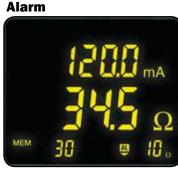
Indicates voltage/current alarm threshold along with the direction of impedance
